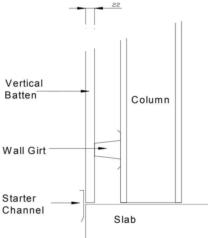
Starter channel is then fixed to the cladding fixing flange with the leading edge of cladding hook a minimum of 35mm below top of slab, using 1 x 10-16 tek per batten. This channel must be level and the accuracy of its level will be reflected in the quality of the finished product. If a constant level mark is created around the entire building you will be able to measure down from that mark to make placement marks for the starter and also a number of the courses of cladding.
